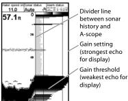
The user can define the level of the weakest and strongest echoes to be shown on the sonar displays, by using the Gain and Threshold settings. See section 4-4 Gain, for more information.
